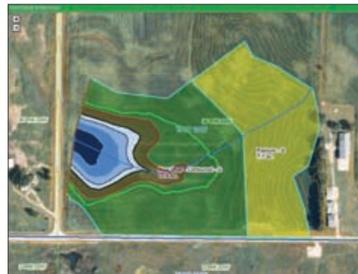
**VISUALIZING WATER DEPTHS:** Screen shots in the WetlandBuilder program are color-coded to show varying water depths that will be created. The shots also show contour lines and where the dike will be. The program will draw a boundary for the wetland's drainage area.
