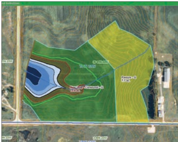
**VISUALIZING WATER DEPTHS:** Screen shots in the WetlandBuilder program are color-coded to show varying water depths that will be created. The shots also show contour lines, where the dike will be, and a boundary for the drainage area of the wetland.
