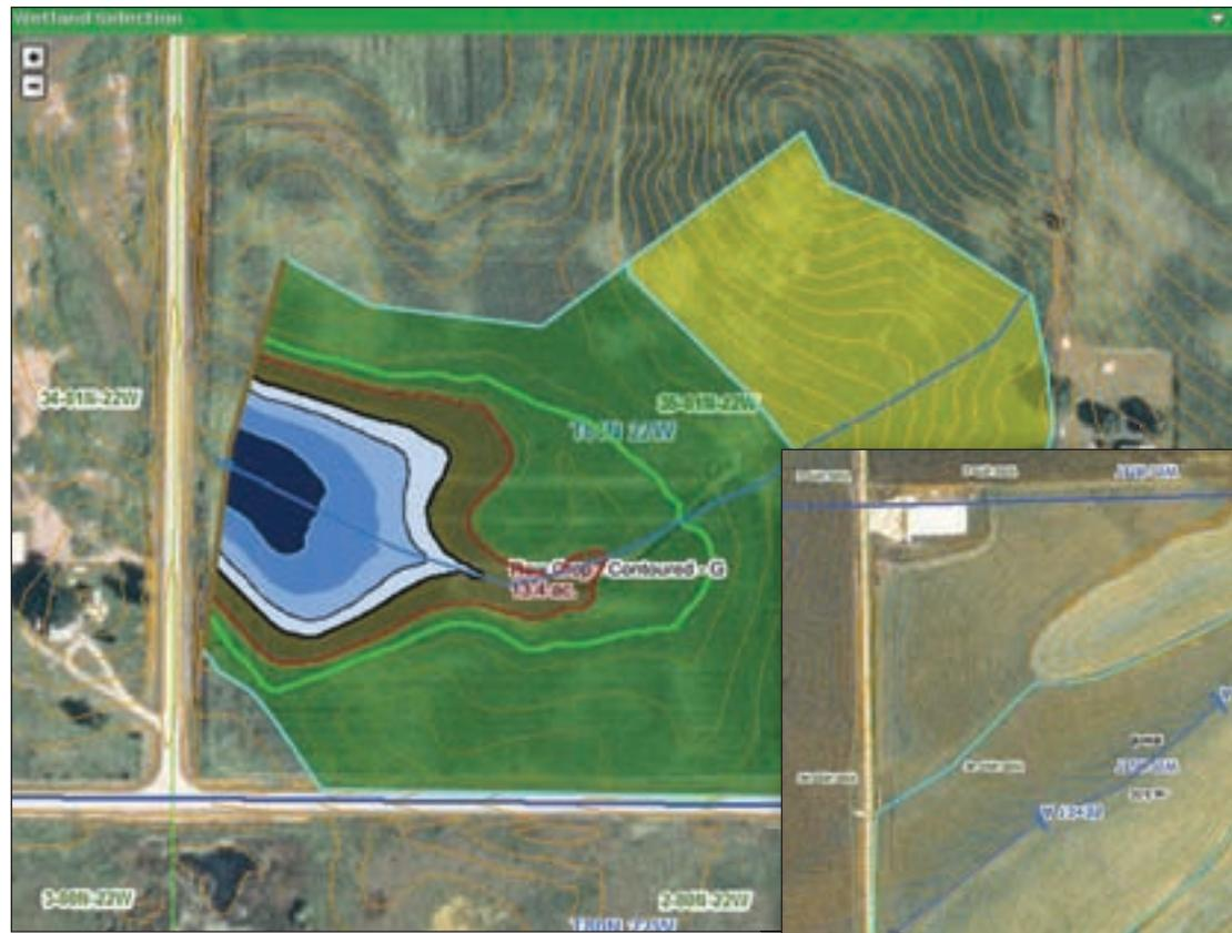
**VISUALIZING WATER DEPTHS:** Screen shots in the WetlandBuilder program are color-coded to show varying water depths that will be created. The shots also show contour lines, where the dike will be, and a boundary for the drainage area of the wetland.
