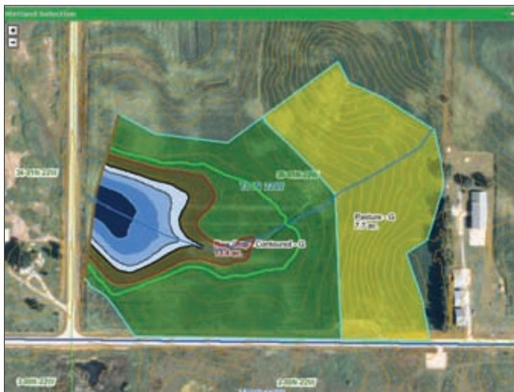
**VISUALIZING WATER DEPTHS:** Screen shots in the WetlandBuilder program are color-coded to show varying water depths. The shots also show contour lines and where the dike will be, and draw a boundary for the drainage area of the wetland.
