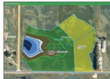
**VISUALIZING WATER DEPTHS:** Screen shots in the WetlandBuilder program are color-coded to show the varying water depths that will be created. The shots also show contour lines and where the dike will be, and they draw a boundary for the drainage area of the wetland.
