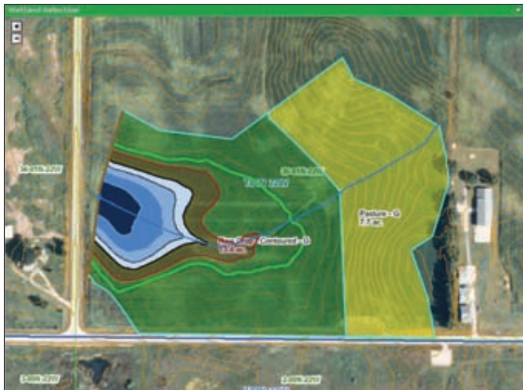
VISUALIZING WETLAND WATER DEPTHS: Screen shots in the WetlandBuilder program are color-coded to show the varying water depths that will be created. The shots also show contour lines and where the dike will be. The program will also draw a boundary for the drainage area of the wetland.
